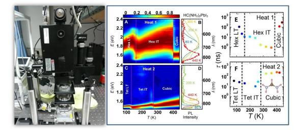
Figure 1 : (left) The Variable Temperature Laser Scanning Conjugate Focus Spectroscopy Microscope built by the Taiwan team. (right) Upon two different heating processes, the temperature-dependent photoluminescence spectra (A, D) and time-resolved photoluminescence lifetime (E, F), when FAPbI3 goes into a cubic phase, significant increases of photoluminescence lifetime are observed upon both processes.
